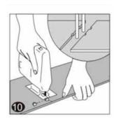
11. Door molding and skirting: Lay a board (with the decorative side down) next to the door moulding and saw as shown in the figure. Then slide the floorboard under molding.
