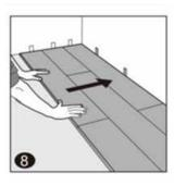
9. To lay the last row: Position a loose board exactly on top of the last row laid. Place another board on top, with the tongue side touching the wall. Draw a line along the edge of this boards, to mark the first board. Cut along the edge of this board to mark the first board. Cut along this line to obtain the required width. Insert this cut board against the wall. The last row should be at least 50mm wide. The spacers can then be removed.
